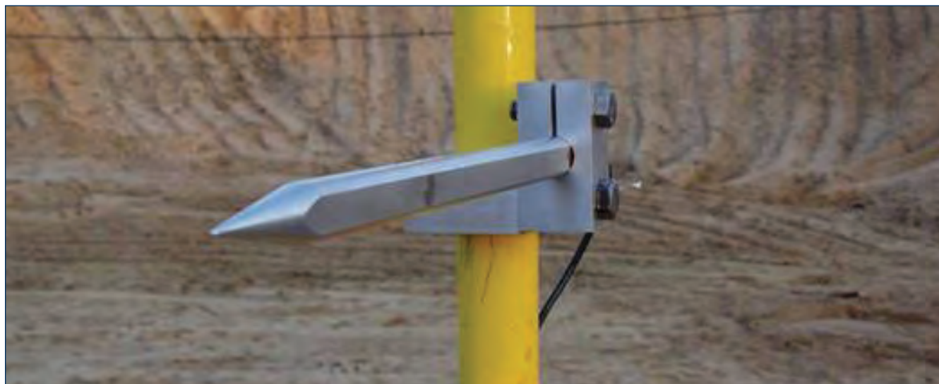
Photo 2: Typical mounting of a Pencil Probe.
